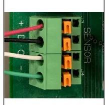
It comes with 15 feet of wire. If more length is required, up to 50 feet of 18 guage thermostat wire may be used. No shielding is required. Connect to terminals on the upper left side of the circuit board labeled Sensor
