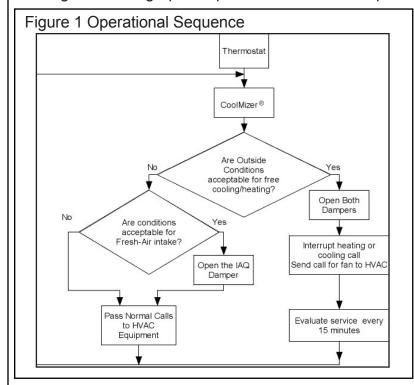
Service Change-Over: Once CoolMizer® starts the equipment, it continues to serve that call with the equipment until it is satisfied. If the call is initially served with outside air, a 15-minute timer is started. At the end of 15 minutes, CoolMizer® reevaluates outdoor conditions to see if they are still within the prescribed parameters.
