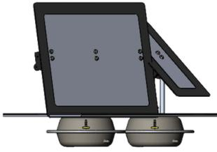
The Damper2™ damper has been designed to control two levels of airflow with one convenient package. The larger portion of the damper brings in larger volumes of air for free heating or cooling. The smaller window brings in a lesser amount of air for controlled ventilation and IAQ. The amount of air brought in is controlled by the size of the total opening and the relative sizes of the damper portions.
