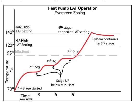
This graph shows how the heating LAT system operates. If the LAT Sensor reading exceeds its set-point, the panel stages down one stage. If the temperature remains above the setting for three more minutes then it stages down again. For all-electric units the system will stage down through all four stages of heat (W2,W1,Y2,Y1).
