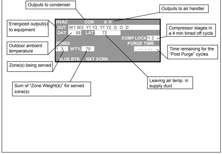
The Evergreen Zoning System provides some very useful information that makes troubleshooting simple. The Evergreen Zoning System has the ability to detect input signals from zone thermostats that do not make sense and provide a visual "ILL" (illegal) call indicator on the LCD screen.
