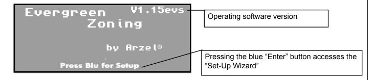
The LCD screen on the Evergreen Zoning System provides a simple way to view system operations. Once the operating parameters are set in the Set-Up Wizard, the LCD display will default to the "Main Operations" screen shown below.
