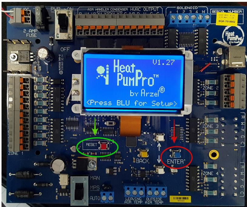
To turn on the LCD display for the first time, push the red **"Reset"** button on the board just beneath the LCD display.
