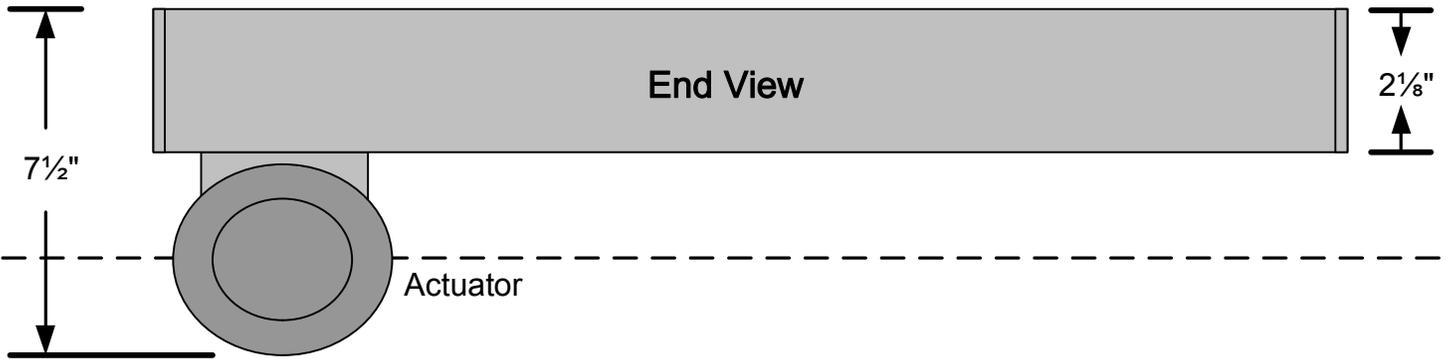
Damper will be built 25" less than nominal size unless specified by "Exact Dimension"
