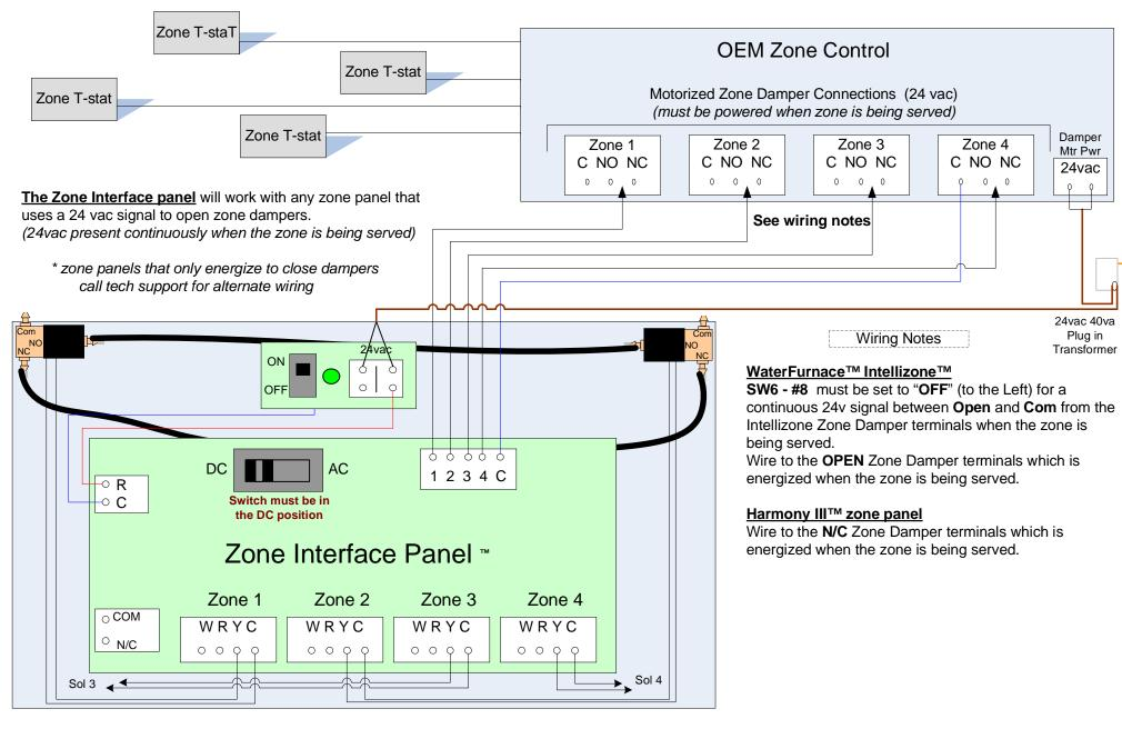
Description: Zone Interface Panel Installation wiring
