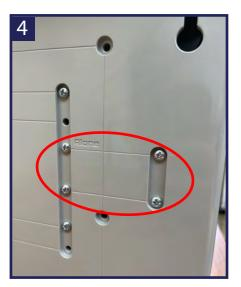
Use the remaining four screws to mount the four provided plastic standoffs. Place the screws in the four holes labeled "Alone" on the back of the panel.
