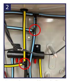
Cut into the existing blue and yellow tubing trees and insert the provided tees with blue and yellow tubing. These tubes will run from the provided solenoid to the existing yellow and blue tubing ladders.
