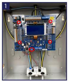
Remove the panel from the wall. Unscrew the two red wires for the pump from the main circuit board. Remove the 1/4 in. hex nuts that mount the board in the panel and lift the circuit board off the standoffs.
