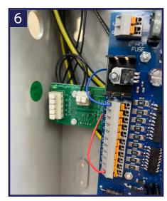
Follow the wiring diagram on the next page to connect wires as needed. Then re-mount the main circuit board, and complete the wiring as shown. The supply air temperature sensor must be mounted in the supply duct for the Smart Zone to operate. The sensor must be located in the supply trunk, placed near the equipment before any dampers, branch runs, or bypass. If additional wire length is required, thermostat wire can be added.
