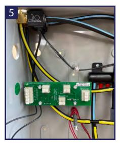
Mount the provided circuit board onto the newly mounted plastic standoffs. Use the four provided 1/4 in. hex nuts to fix the circuit board in place.
